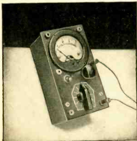
The Ya Mei multitester. Test leads are shown in the D.C. jacks.
