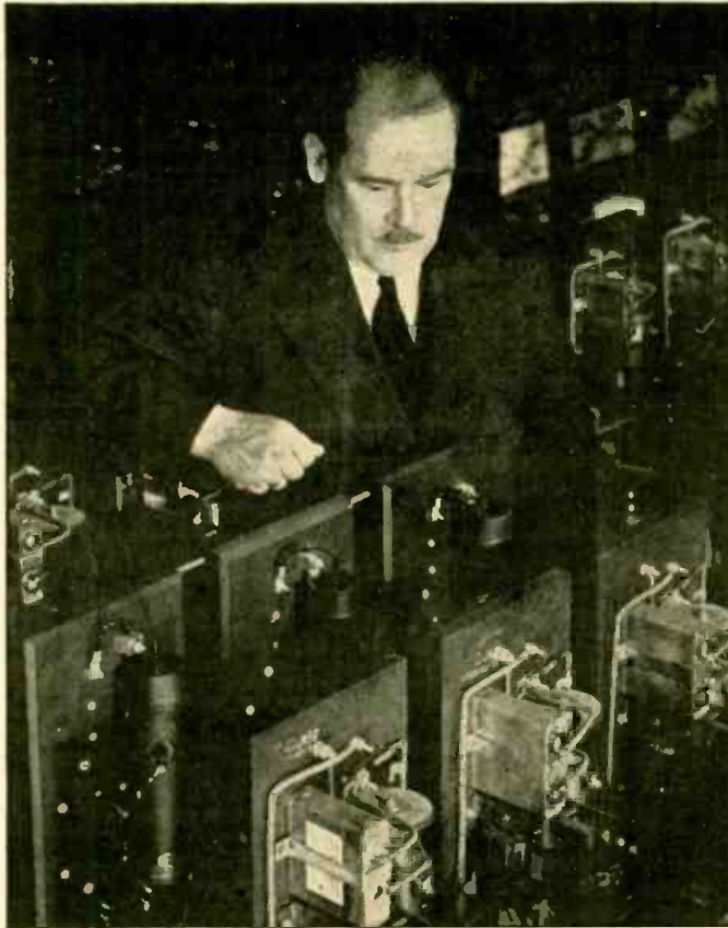
Dr. E. F. W. Alexanderson, G.E. Consulting Engineer, in his laboratory, shown with test set for Thyatron power circuits. Three small metal Thyatron tubes shown on panels immediately in front of him.
